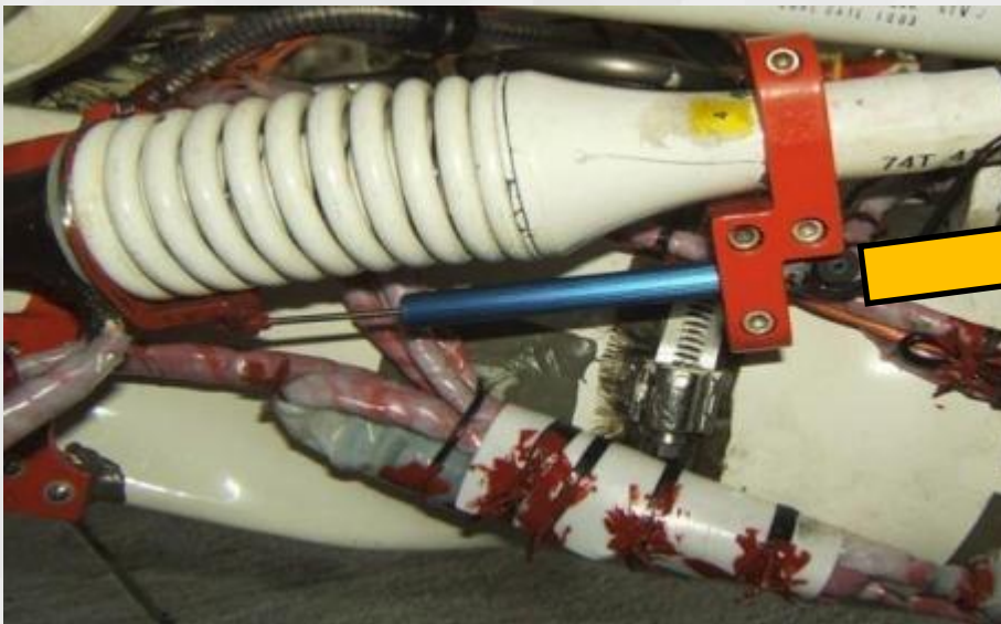
Aircraft left planning link spring displacement sensor on the main landing gear.
